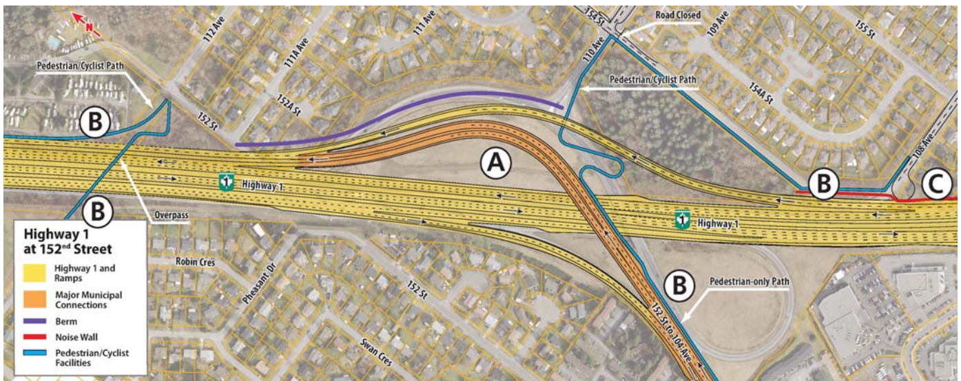
A map of the final configuration at 152 Street, including a new, reconfigured on-ramp, new local connection lanes, pedestrian/cyclist paths, noise walls and berm.
