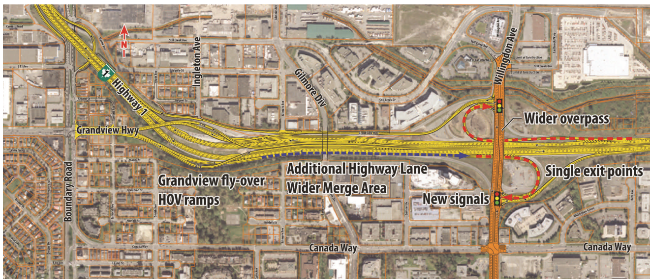
This graphic of the new configuration shows all traffic exiting at Willingdon routed under the overpass before proceeding to traffic signal-controlled intersections at Willingdon. This configuration will dramatically reduce traffic weaving and congestion in the area and improve safety.
