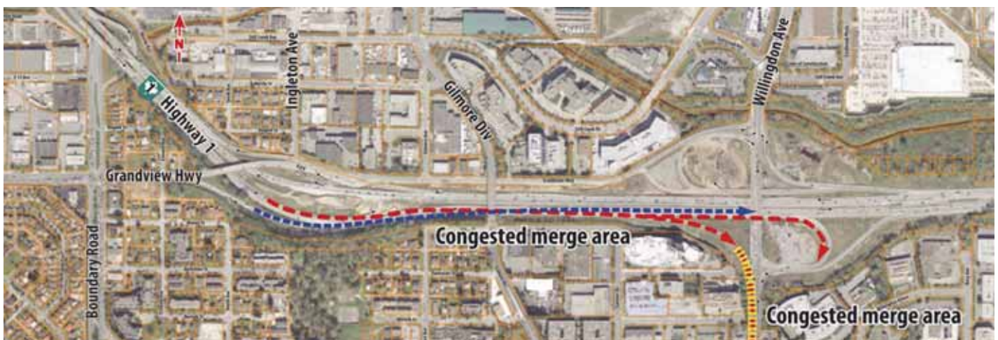
This graphic of the current configuration shows the limited space between the Grandview Highway on-ramp and the Willingdon Avenue Interchange. This configuration can lead to increased congestion and contributes to a high accident rate for the area.
